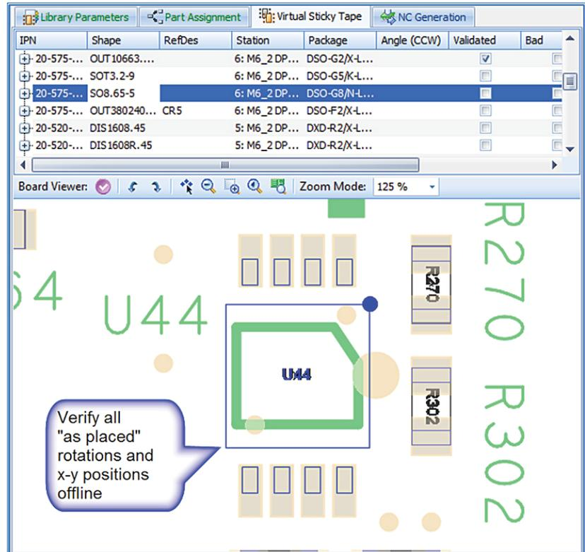
*Eliminate line downtime from program errors with Virtual Sticky Tape. This simulation feature allows for "as built" component rotations and offsets to be verified offline in a virtual simulated environment for right first time production.*
