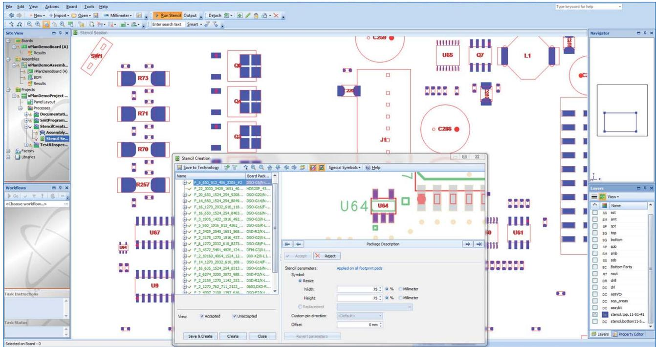
With Valor MSS Process Preparation, you can design your own stencils, streamlining the process and reducing errors. Output can be either ODB++ or 274X Gerber files.
