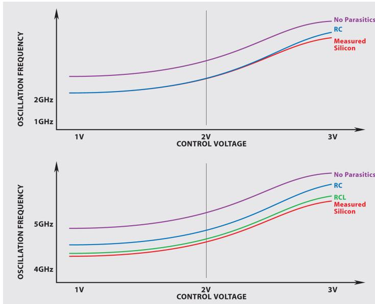
Parasitic inductance (noise, distortion, impedance mismatch and jitter) can cause chip failure if not accounted for in parasitic extraction. At higher frequencies, inductance can shift the frequency of oscillation in a VCO (lower graphic) and must be taken into account.
