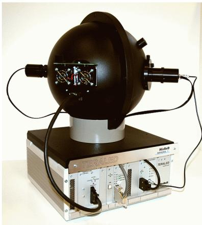
**Figure 6:** An automated photometric/radiometric measurement setup with a Peltier-cooled LED fixture, used in connection with the T3Ster thermal transient tester
