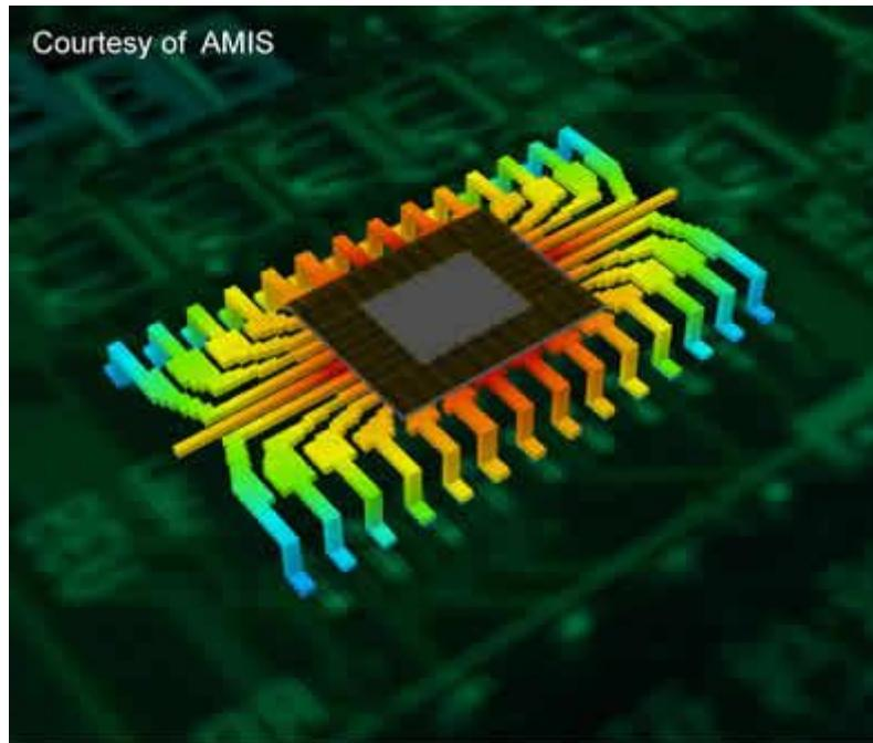
AMI Semiconductor (AMIS) is using Flotherm and Flopack in the design and development of ASICs for automotive, medical, industrial, communications and consumer applications. This example shows a detailed thermal analysis including the silicon die, die flag and leadframe of a 28-lead Small Outline Integrated Circuit (SOIC) package.
